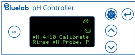
ready for pH 4 or pH 10 calibration
