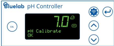
successful pH7 calibration
