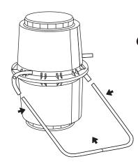
**5** Fit one leg set to elbows by pressing "U" shape together sufficiently to allow entry to elbows.
