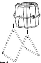
Connect the assembled compost tumbler body(assembled from step 3) to the legs(assembled from step 2) with 2 L screw sets(#5)
