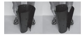
4. Pull the third section outwards to complete the circle at the wide end and firmly lock the lug closest to you (the one at the top) into the adjacent receptor hole.
