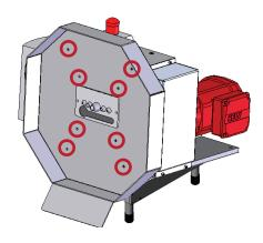
STEP 2: REMOVE FRONT **CUT PLATE**
