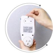
Secondly, put it into the power supply, the LCD screen of the power meter will show and will last for about 3 seconds.
