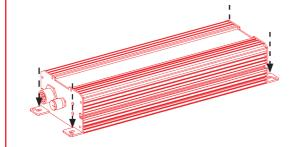
Mount driver to a secure surface with screws.
