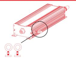
**1.** Slide and tighten eyebolts in driver channel.
