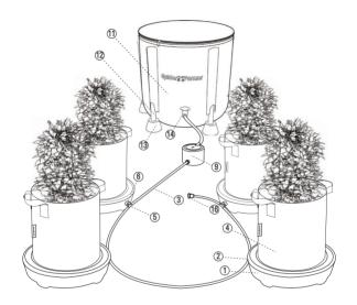
**Step1**: Open the Shut-off Valve Box(§), remove the cotton pad, and then close the Shut-off Valve Box cap.
