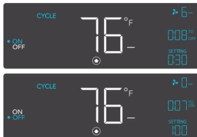
If there is a speed set in OFF Mode other than zero, the fans will run at that speed when triggered to turn off.
