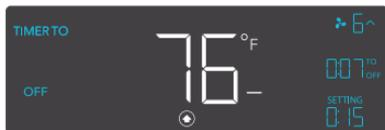
If there is a speed set in OFF Mode other than zero, the fans will run at that speed when triggered to turn off.
