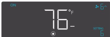
Do not set this level to zero, as this will result in the fan not activating when triggered ON.
