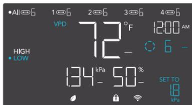
Either of the two trigger points can activate while you are in VPD Mode, even if you are viewing another trigger point. Set a trigger point to OFF if not in use, by holding down the up and down button. If there is a level set in OFF Mode other than zero the devices will run at that level when triggered to turn off.
