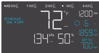
If there is a level set in OFF Mode other than zero, the devices will run at that level when triggered to turn off.
