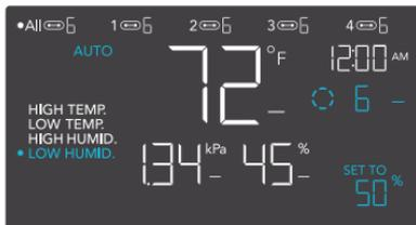
Any of the four trigger points can activate while you are in AUTO Mode, even if you are viewing another trigger point. Set a trigger point to OFF if not in use, by holding down the up and down button. If there is a level set in OFF Mode other than zero the devices will run at that level when triggered to turn off.
