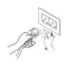
After turning the unit off, please take plug out of the socket.
