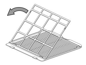
Clean the filter using a slightly damp, soft, lint-free cloth. If the filter is heavily contaminated, clean it with warm water mixed with a neutral cleaning agent.
