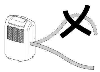
Remove the hose if you want to collect the condensate in the condensation tank again. Allow the hose to dry prior to storage. The hose can be connected in any operating mode for continuous operation.
