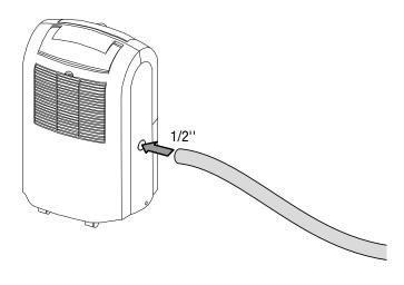
Check whether the hose is properly positioned on the connection. If necessary, adjust the position through the condensation tank opening.
