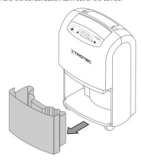
2. Empty the condensation tank over a drain or sink.
