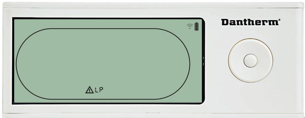
Dehumidifier stopped because of Low Pressure detection.
