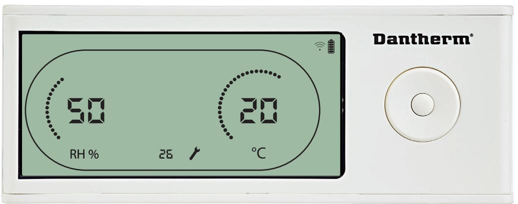
While flashing, the service interval can be increased by pressing RIGHT Button or decreased by pressing the LEFT Button.
