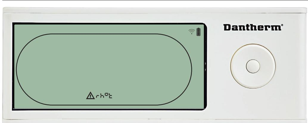
If RH/T sensor is defect, then "rh°t" code will be shown when pressing UP or DOWN during screen shows Sensor fail code "SEnS".
