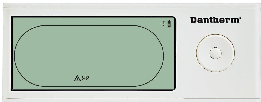
Dehumidifier has stopped because of High Pressure detection.
