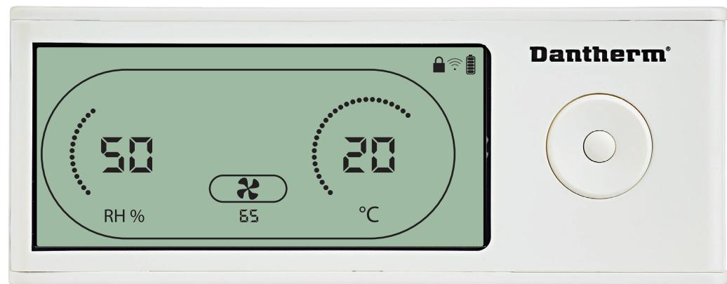
When the extractor fan icon flashes at 0.5 Hz and extractor fan set point value is shown on info line.
