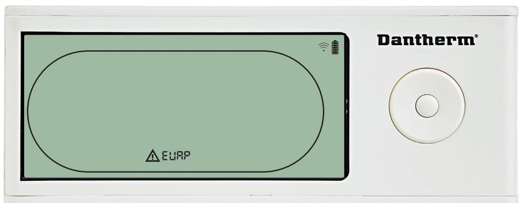
If evaporator sensor is defect, then "EVAP" code will be shown when pressing UP or DOWN during screen shows Sensor fail code "SEnS".
