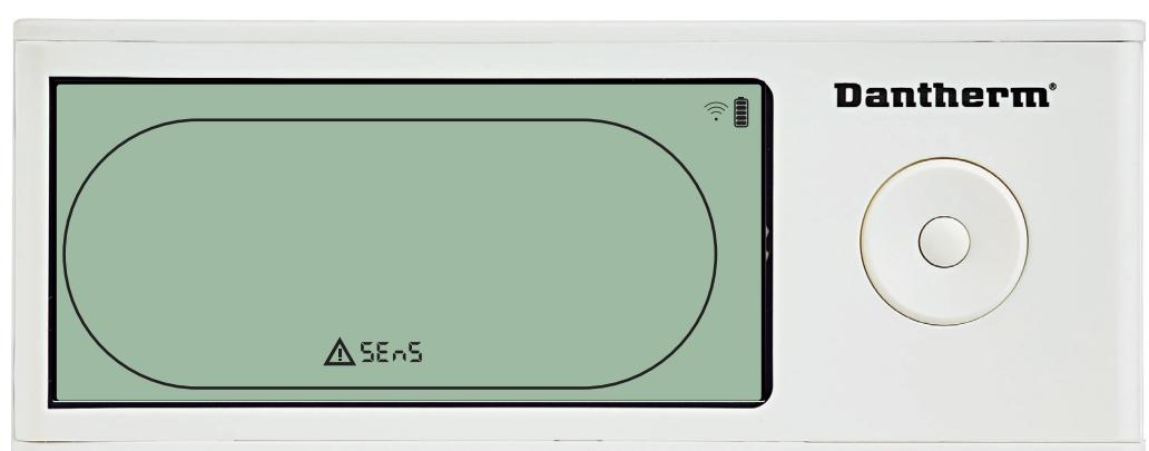
Dehumidifier is stopped because sensor failure is detected. Sensor Fail can not be dismissed from DRC1. Use UP or DOWN button to see which sensor/sensors are defect If all sensors are defect these codes show in the following sequence: "COnD" ↑ "EVAP" ↑ "RH/T" It is not possible to enter menu setup to modify set point values
