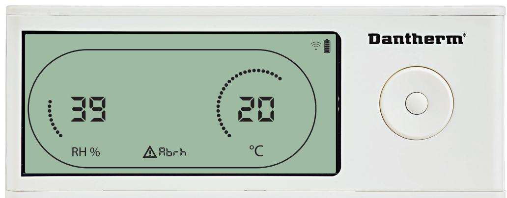
DRC1 enters stand-by mode 2 when ambient conditions are out of operation range. The display will show temperature and Rh readings when the unit is in stand-by mode 1. This state will only get corrected when the ambient temperature (abt) or ambient humidity (abrh) is in range, and can not be dismissed. You can enter menu setup to modify set point values – only in this case. While in Menu Setup, the alarm icon turn off and set point value will be shown instead of "Abt/Abrh" code on INFO line
