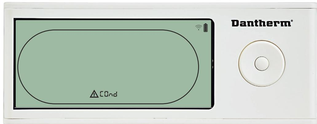
If condenser sensor is defected, then "COnD" code will be shown when pressing UP or DOWN when screen shows Sensor fail code "SEnS". If no buttons pressed within 10 seconds then screen will again show "SEnS" again. It is not possible to enter menu setup to modify set point.
