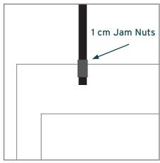
ATTENTION: Threaded rods should be engaged no less than 3.8 cm into machine, and no greater than 6.4 cm.
