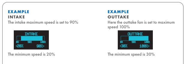
In this example, minimum speed of the outtake will be 10% faster, and at maximum speed the outtake will be 10% faster.
