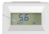
Successful pH 7 and pH 4 calibration
