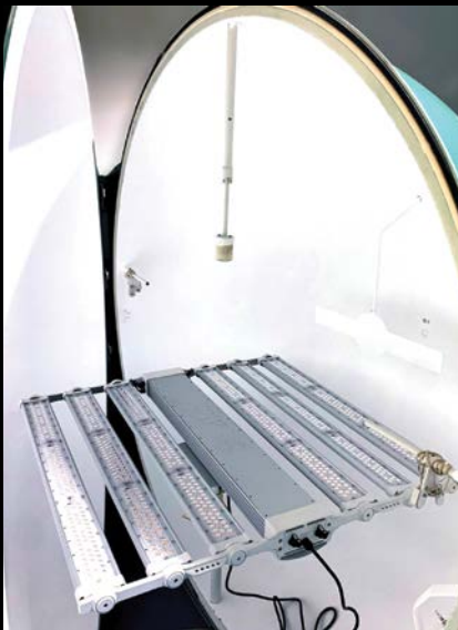
Lab testing example with an integrated sphere that closes and measures the entire photon output of the fixture.
