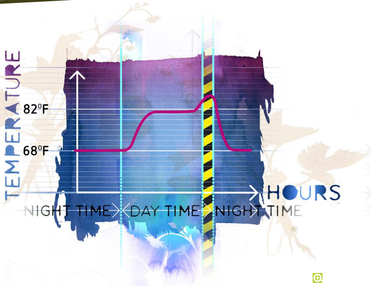
Figure 3: Infra-red thermometers, and dataloggers are the tools of choice when you are wanting to correctly monitor the VPD. A spike in air temperature on the graph (usually towards the end of the day(lights on)) will indicate closed stomata. Dimming lights is an easy solution for this problem, though the root cause will still need addressing.
