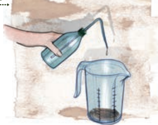
Add demineralised water to the sample until the soil is saturated.
