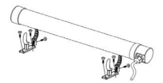
**Step 2.** Fix the tube heater on the wall or on the floor as shown in above diagram.
