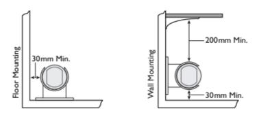
**Step 1.** Install the bracket as shown in above diagrams.
