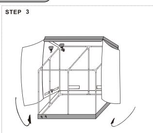
Then pull the bottom of tent shell to cover the base of tent frame propertly. Put all hanging bars on the top of frame.
